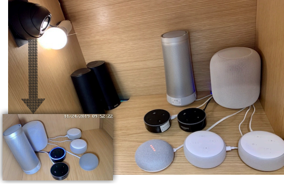
Fig. 1. Testbed: camera and light to capture activations (top left), speakers controlled by us to play audio content from TV shows (center left), smart speakers under test (right). The bottom left shows the frame of an activation, i.e. , an Echo Dot device lighting up, as detected by the camera.
